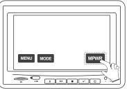
To power the off unit, press MPWR or PWR on the monitor; or press POWER button on the remote control.
